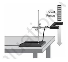
Determine experimentally the gravitational acceleration constant " $\vec{q}$ "
