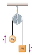
To solve it, let's separate the system into two smaller systems, where each system consists of one mass, and apply Newton's second law for each system. Since the movement of each object is just in the vertical direction, we only need to calculate the net force in the "y" direction for each object.
