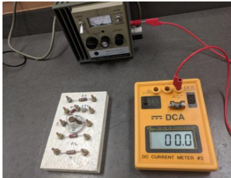
Figure 3 With units off, connect a red wire from the + terminal of the power supply to the 250 mA (max) + terminal of the ammeter.
