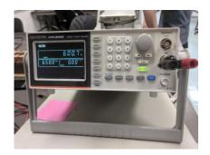
i) Ensure that the unit is plugged in AC power. Press in the power switch in the lower right. Connect a BNC to Banana adapter to the MAIN Output 50  $\Omega$ , second from the top on the right.
