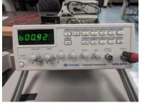
i) Ensure that the unit is plugged in AC power. Press in the power switch in the lower left. Connect a BNC to Banana adapter to the **Output 50**  $\Omega$ , in the lower right.
